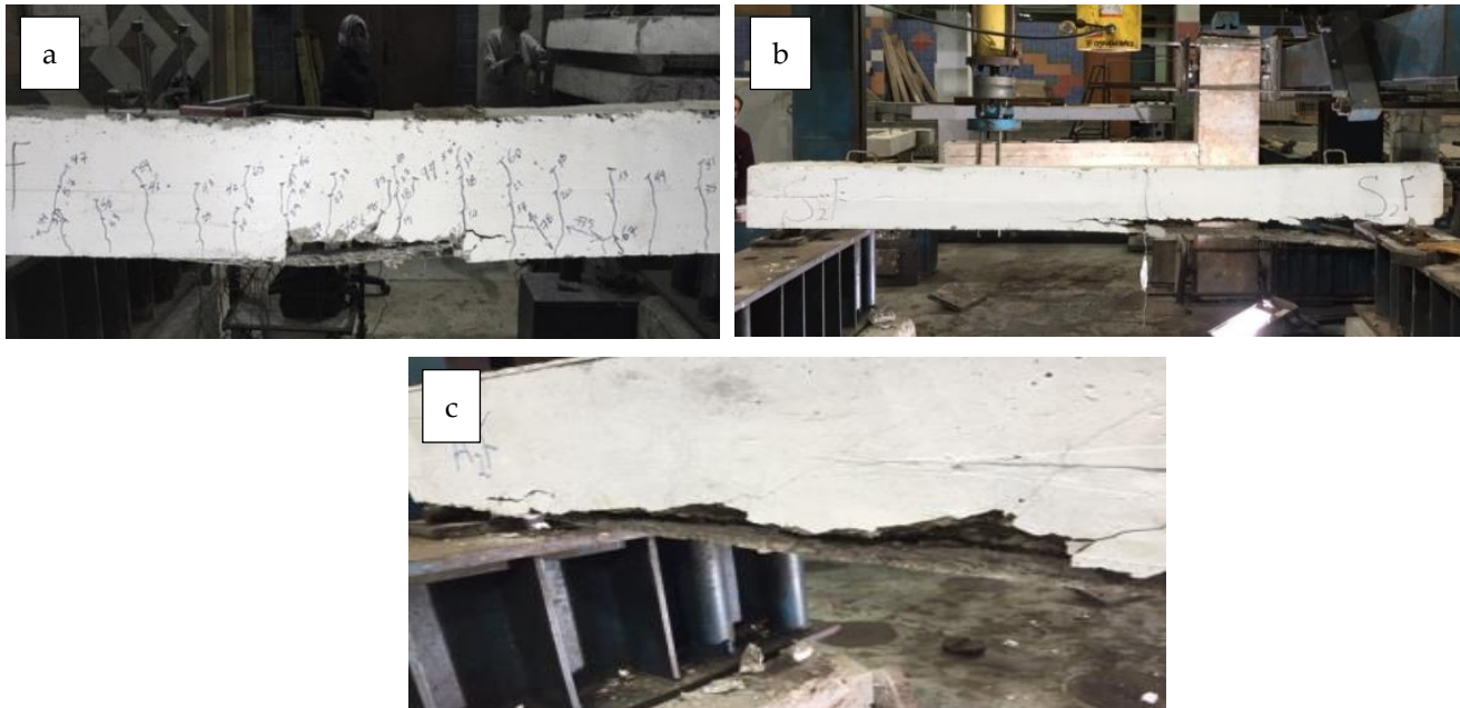
Figure 2. Failure modes of the tested beams (a) Beam S1F, (b) Beam S2F and (c) Beam A2F
